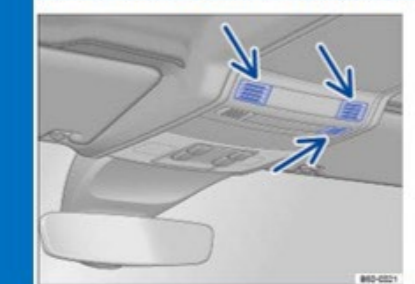
Interior monitoring system and anti-tow alarm
